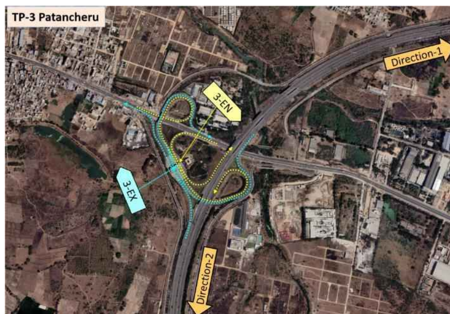
Figure 2-7 : Double Trumpet Type Interchange
