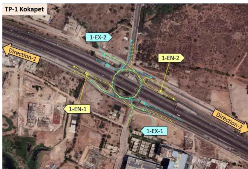
Figure 2-5 : Rotary Type Interchange with 4 toll booths.
